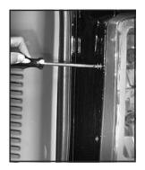
Use a screwdriver to remove the two screws from the lamp assembly.
